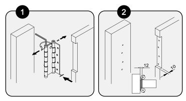
Easy 2 step installation process. Step 1, cut rebate into door, insert allen key into head of hinge remove pin, turn to release tension, reinsert pin. Step 2, screw hinge to door & wall jam, readjust tension. Easy. You're done.
